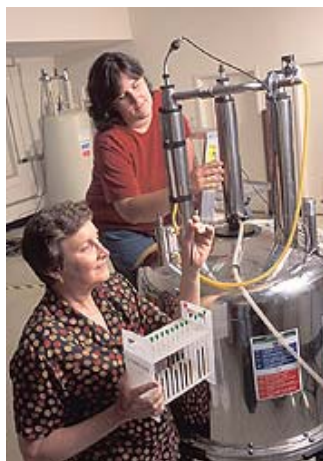
Soil scientist Sara Wright (foreground) and technician Kristine Nichols use nuclear magnetic resonance to examine the molecular structure of extracted soil organic matter constituents. (K9971-1)
