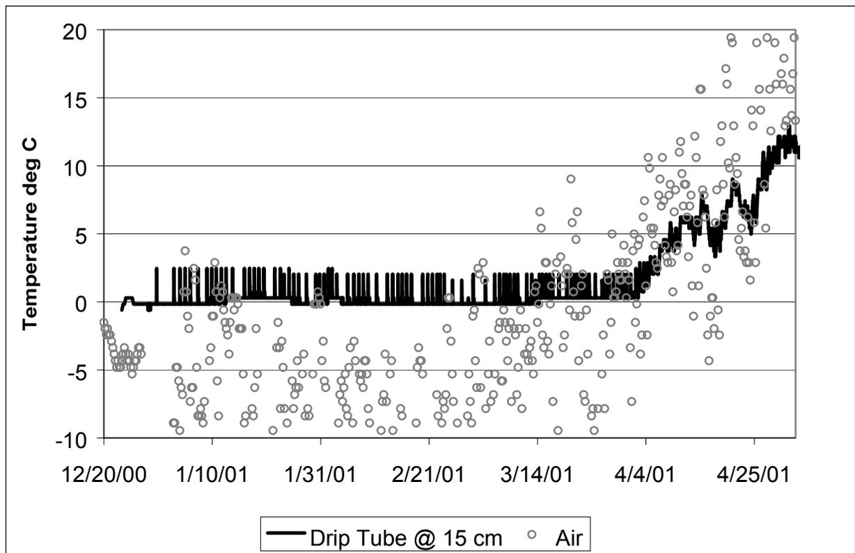
Figure 4. Columbus Elementary School. Temperature of the Emitter lines with 15 cm of Soil Cover.
