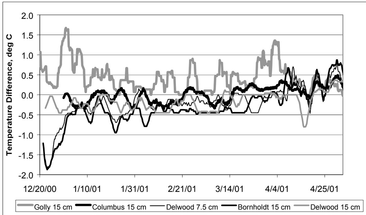
Figure 7. Temperature Difference Between the Emitter Line and the Soil Between the Emitter Lines. (Negative numbers indicate the emitter line is colder than the soil between emitter lines. Data presented is a running 3-day average of logged temperature readings).
