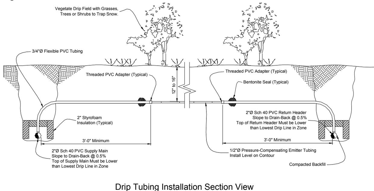
Figure 6. Recommended Configuration of Supply Mains and Return Headers to Avoid Freezing of Emitter Lines.
