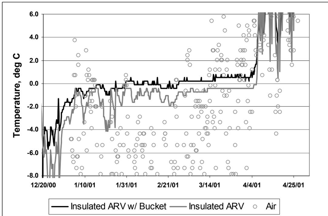
Figure 9. Performance of Valve Box Insulation Designs.
