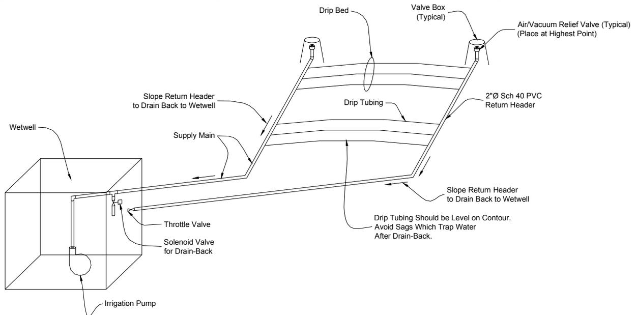
Figure 1. NAWE Cold-Climate Drip System Schematic.
