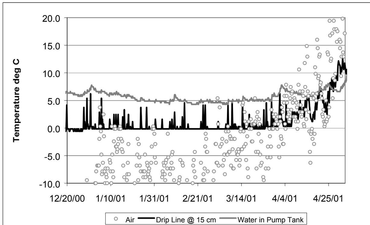
Figure 5. Golly Residence. Temperature of the Emitter Lines with 15 cm of Soil Cover. (Note temperature “spikes” representing dosing events. Temperature during dosing events closely matches the temperature of the effluent in the pump tank.)
