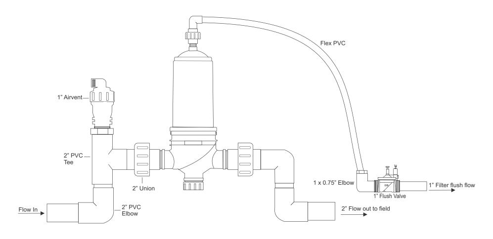
Mount/affix to a base or to the floor of the building. Can be strapped or buried. Note: If unit is inside a building, be sure to include a drain on the building floor.
