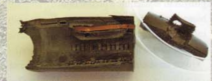
Figure 5: The Adi Rootguard® dripper with no root intrusion or accumulation of clogging matter at the inlet filter, the water passageway, or the emitter outlet.
