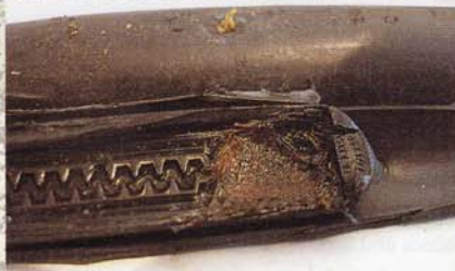
Figure 1: A dripper without RT blocked by root intrusion, clogging the emitter's outlet and the inner water passageway.
