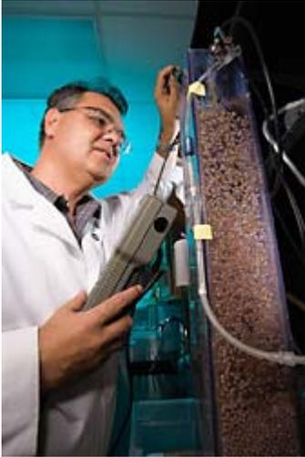
Soil scientist Matias Vanotti monitors conditions in a bioreactor that uses immobilized bacteria to remove nitrates from agricultural effluents. **(D1316-1)**
